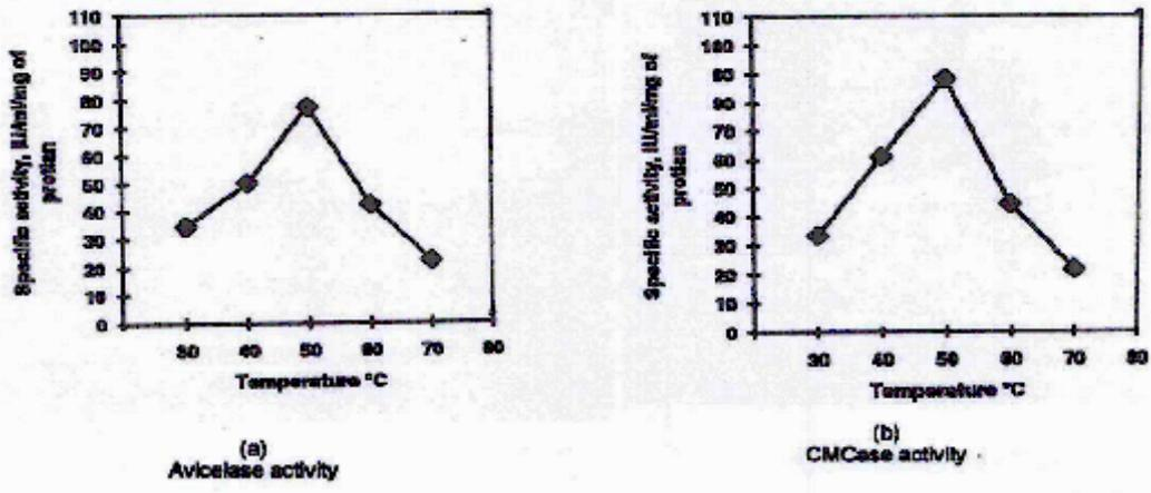
Fig. 6. Temperature optima for Avicelase and CMCase enzymes
