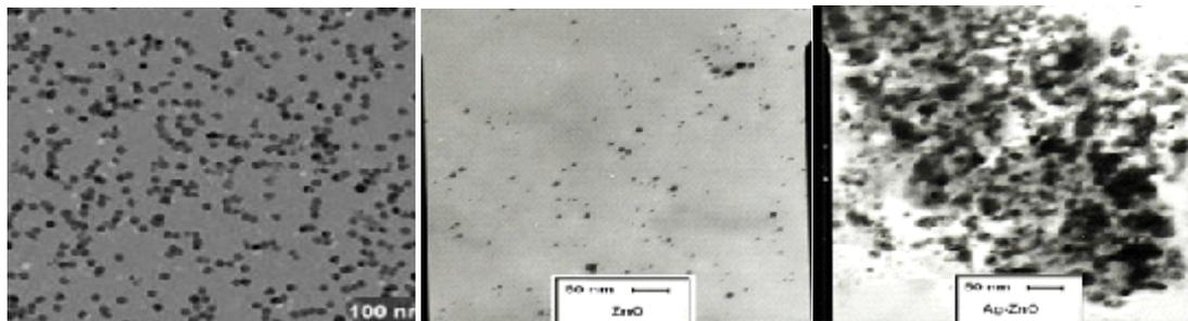
Fig. 3. TEM images of (a) Ag, (b) ZnO and (c) Ag/ZnO nanoparticles
