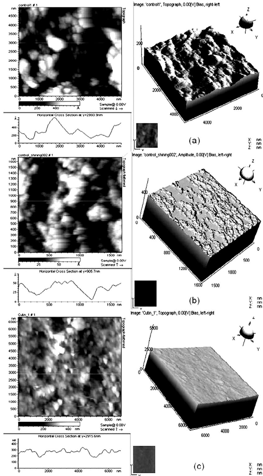
Fig. 1. AFM image of (a) untreated tomato peels (b) enzyme treated tomato peels and (c) Cutin.
