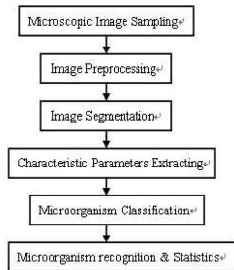
Fig. 1. The designed the structure of water microorganism classifier
