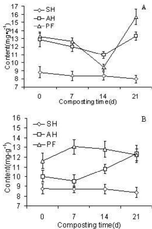
**Fig. 3.** Changes of different components contents in compost over time. A: treatment 2. B: treatment 5. SH: saturated hydrocarbon; AH: aromatic hydrocarbon; PF: polar fraction. Values are expressed as means±SD( $n=3$ )
