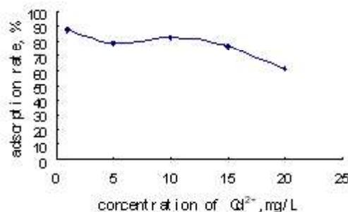
Fig.4. Biosorption of  $Cd^{2+}$  at different initial concentration
