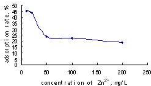
Fig. 3. Biosorption of  $Zn^{2+}$  at different initial concentration
