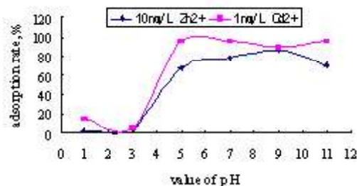
Fig. 5. Effect on  $\text{Zn}^{2+}$  and  $\text{Cd}^{2+}$  sorption at values of pH
