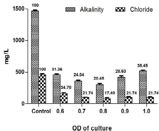
Fig. 3. Alkalinity and chloride reduction of cement kiln dust (CKD) treated with different concentration (in terms of optical density) of *Bacillus* sp. strain KG4. The numbers on the bars represents the percent alkalinity and chloride, respectively, in different treated CKD samples compared to untreated CKD (control). Statistical analysis shows  $p < 0.05$  using t-test at 95% confidence limits
