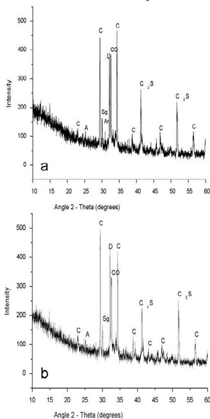
**Fig. 4.** Diffraction pattern including the crystalline phases in the control CKD (a) and bacterial treated CKD (b). C-calcite ( $\text{CaCO}_3$ ), D-dolomite ( $\text{CaMg}(\text{CO}_3)_2$ ), A-anhydrite ( $\text{CaSO}_4$ ), CO-calcium oxide (CaO), Sg-syngenite ( $\text{K}_2\text{Ca}(\text{SO}_4)_2$ ), Ar-arcanite ( $\text{K}_2\text{SO}_4$ ) C2S-dicalcium silicate, C3S-tricalcium silicate
