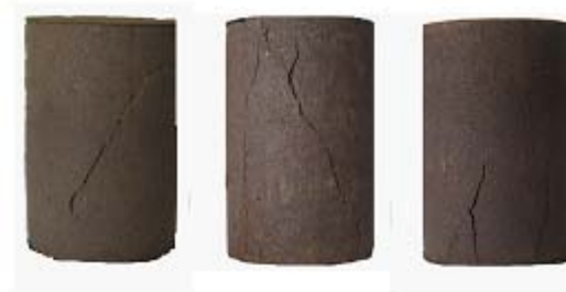
Fig. 4. The damage form of soil sample
