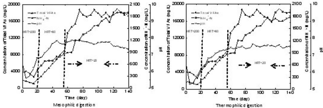
**Fig. 3.** Evolution of total VFAs, NH<sub>4</sub><sup>+</sup>-N and pH for of Dry anaerobic Mesophilic and Thermophilic Digestions
