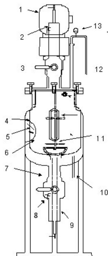
**Fig. 1.** Schematic diagram of experimental set-up(1. Mixing motor, 2. Inlet, 3. Inlet ball valve, 4. Thermocouple, 5. pH meter, 6. Water bath layer, 7. Outlet ball valve, 8. N<sub>2</sub> rectification, 9. Outlet, 10. Water inlet, 11. Mixing blade, 12. Nozzle, 13. Pressure instrument)
