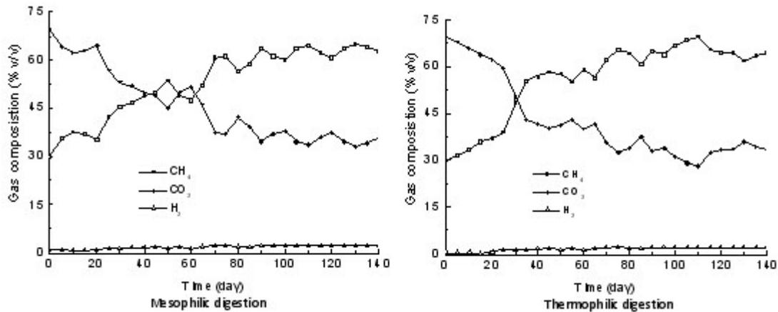
**Fig. 4.** Evolution of gas composition of CH<sub>4</sub>, CO<sub>2</sub> and H<sub>2</sub> for anaerobic Mesophilic and Thermophilic Digestions
