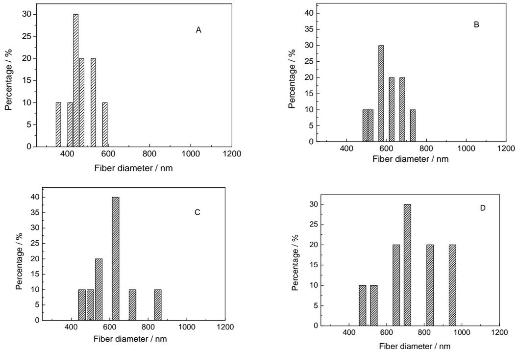
**Fig. 2:** Diameter of PAN/BC nanofibers with different BC contents, (A) 0 wt %, (B) 3 wt %, (C) 5 wt % and (D) 8 wt %
