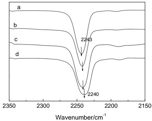
**Fig. 4.** FTIR spectra of the nitrile ( $\text{C}\equiv\text{N}$ ) band in (a) PAN; PAN/BC blends nanofibers with BC content (b) 3 wt %, (c) 5 wt % (d) 8 wt %
