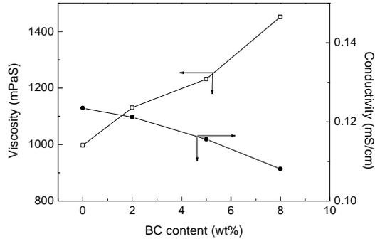
**Fig. 3.** The conductivity and viscosity of electrospinning solution as a function of BC content
