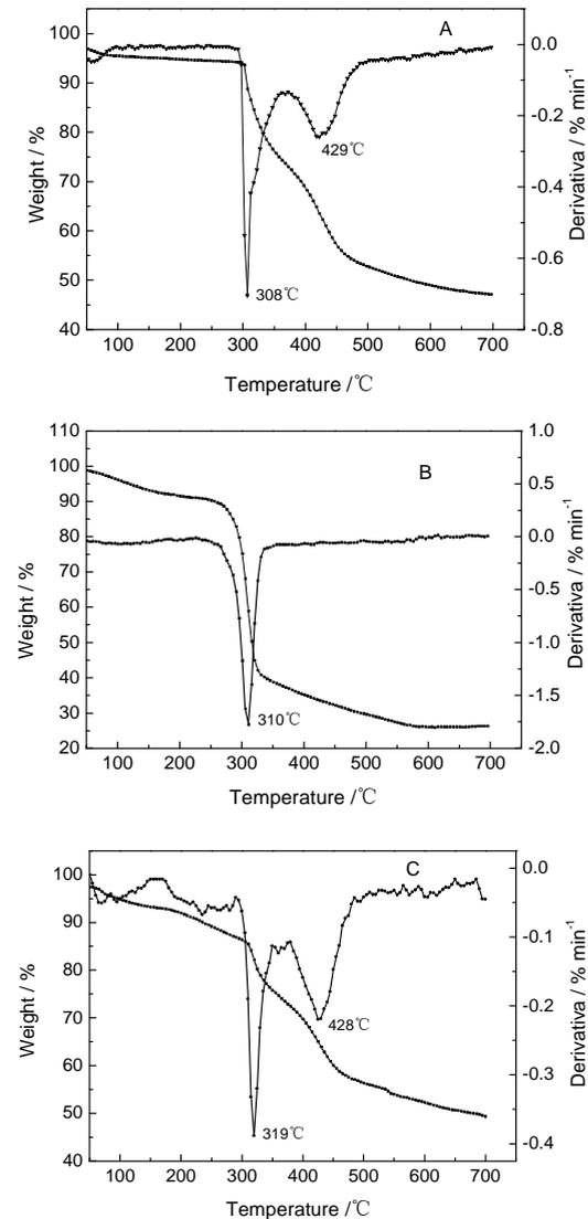
**Fig. 6.** TGA and DTG thermograms of (A) PAN, (B) BC and (C) PAN/BC blend nanofiber with 8 wt% BC
