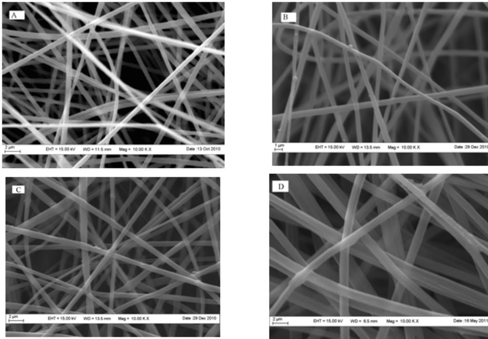
**Fig. 1:** SEM images of PAN/BC nanofibers with different BC contents, (A) 0 wt %, (B) 3 wt %, (C) 5 wt % and (D) 8 wt %
