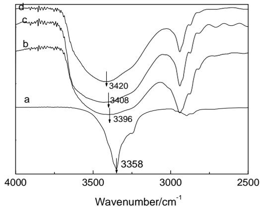
**Fig. 5.** FTIR spectra of the hydroxyl (O-H) group in (a) BC; PAN/BC blends with BC content (b) 8 wt %, (c) 5 wt % (d) 3 wt %
