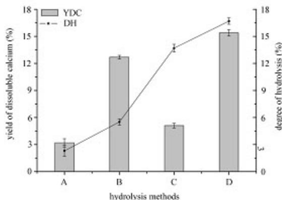
**Fig. 1.** Comparison of four hydrolysis methods. (A) acid hydrolysis; (B) PEF assisted-acid hydrolysis; (C) pepsin hydrolysis; (D) PEF assisted pepsin hydrolysis. Field strengths: 15kV/cm, pulse number: 6, acid content: 0.3mol/L, E/S: 2%. Results are presented as the means ( $n=3$ )  $\pm$  SD. The data mean is significantly different at ( $P<0.05$ )
