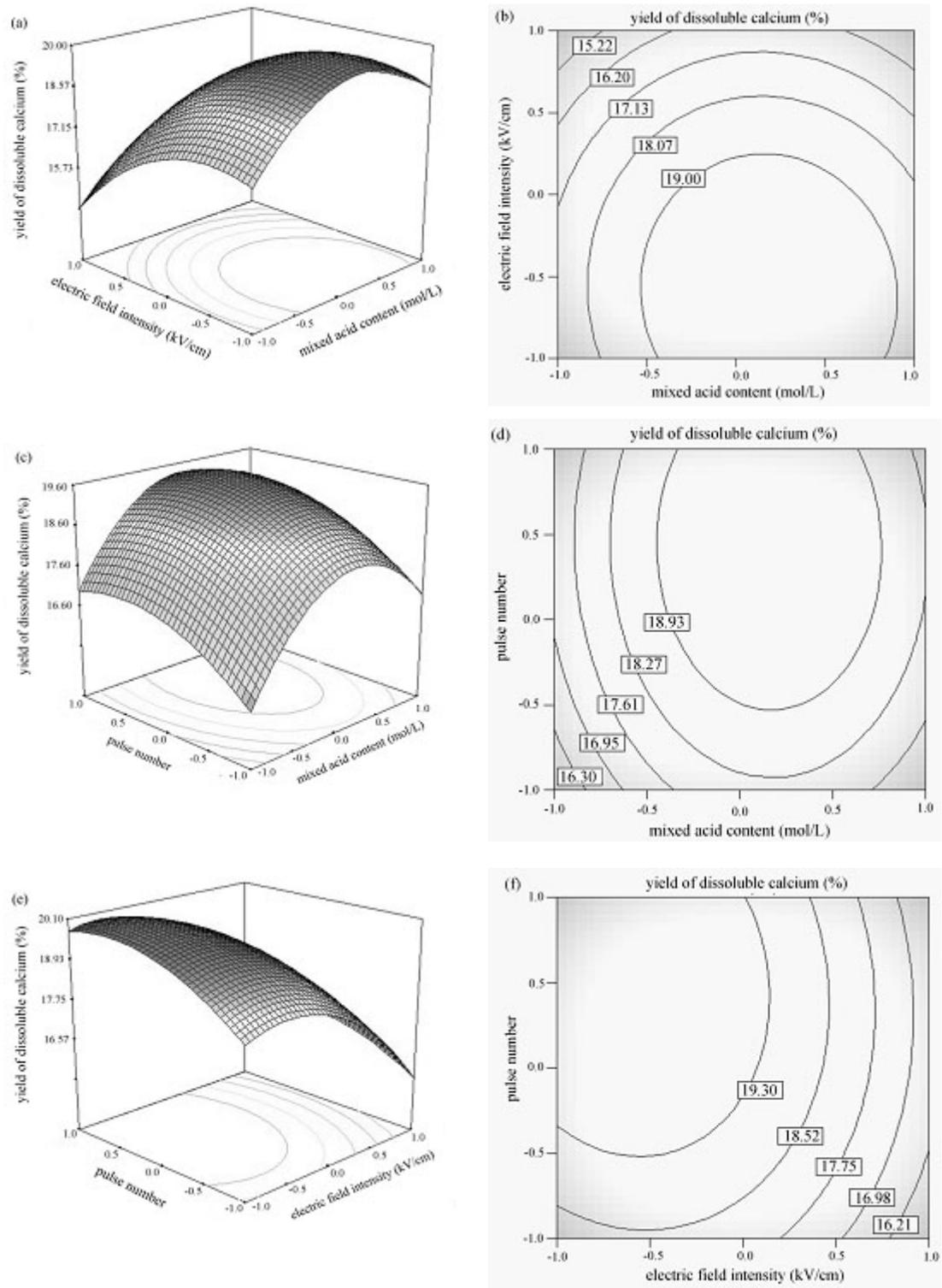
**Fig. 3.** Response surface plots and contour plots of enzymatic hydrolysis reaction. The degree of hydrolysis is shown as a function of the interactions between acid concentration and electric field intensity (a, b), acid concentration and pulse number (c, d), pulse number and field intensity (e, f)
