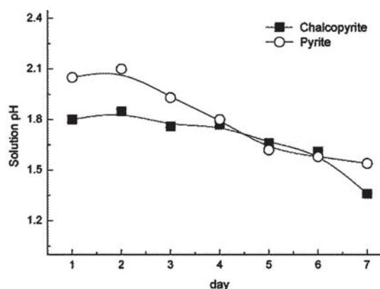
Fig.1. Solution pH evolutions during bacterial adaptation experiments
