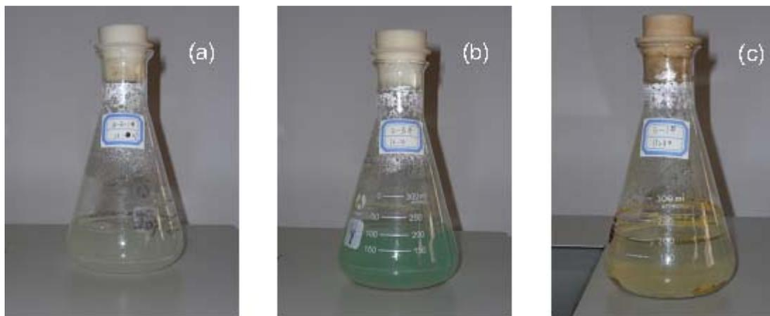
Fig. 2. The appearance after bacterial adaptation for 7 days: (a) controlled sample, (b) sample with chalcopyrite and (c) sample with pyrite
