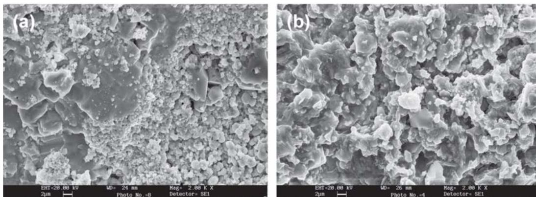
**Fig. 6.** Pyrite surface morphology (a) before and (b) after column bioleaching by extreme thermophilic bacteria: (a) before column bioleaching; (b) after column bioleaching
