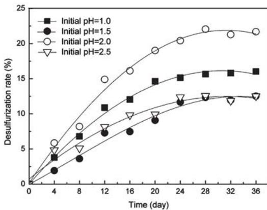
**Fig. 4.** Desulfurization rates throughout the bioleaching by a strain of extreme thermophilic bacteria
