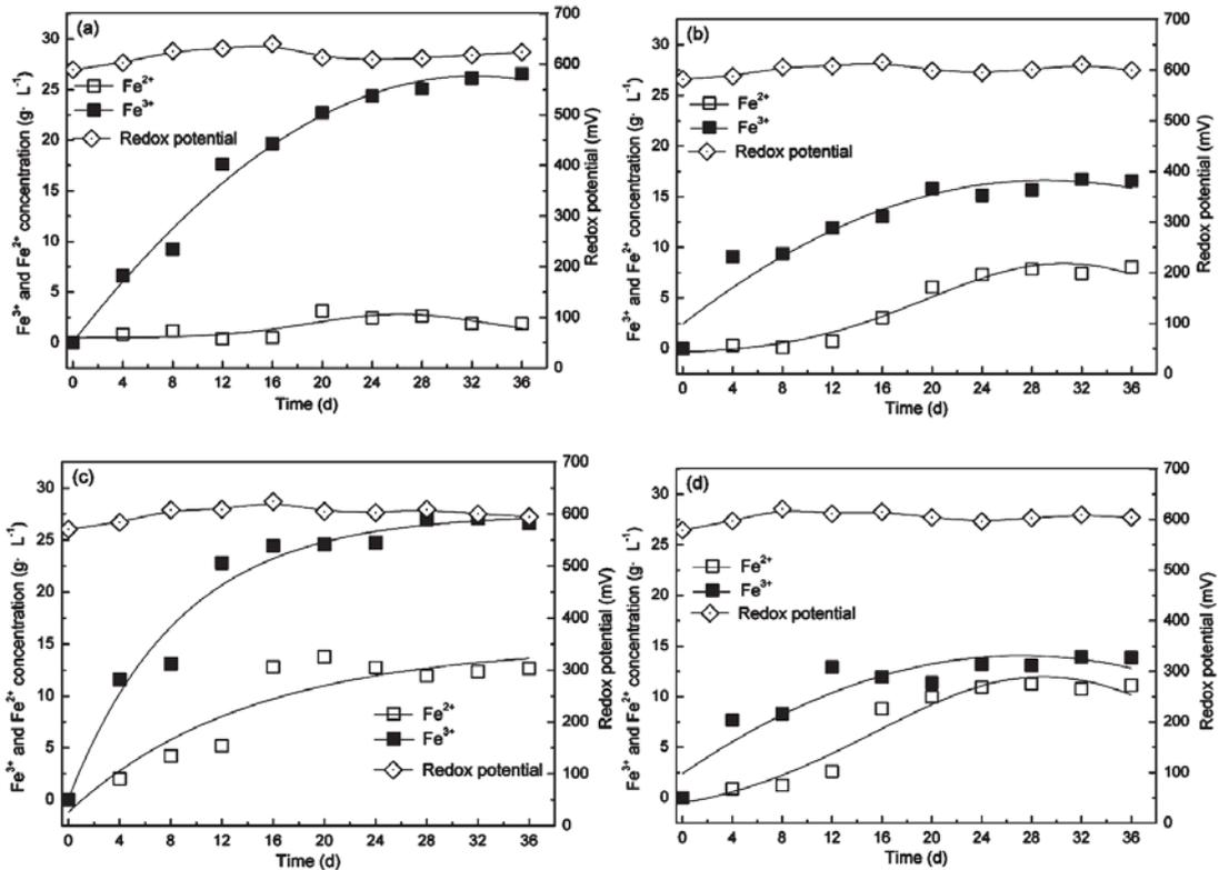
**Fig.3.** Redox potential, Fe(II) and Fe(III) concentration variations throughout the bioleaching process: (a)initial pH=1.0; (b)initial pH=1.5; (c)initial pH=2.0; (d)initial pH=2.5
