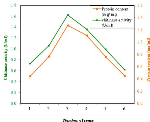
Fig. 8. Semi-continuous production of chitinase by *Bacillus licheniformis* cells adsorbed on carboxymethylcellulose
