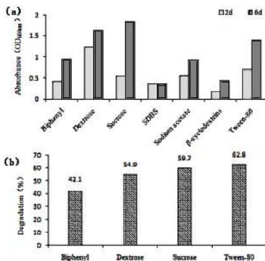
Fig.6(a). Effect of different carbon sources on *PS-11* growth; (b) PCB52 percent degradation on day 6
