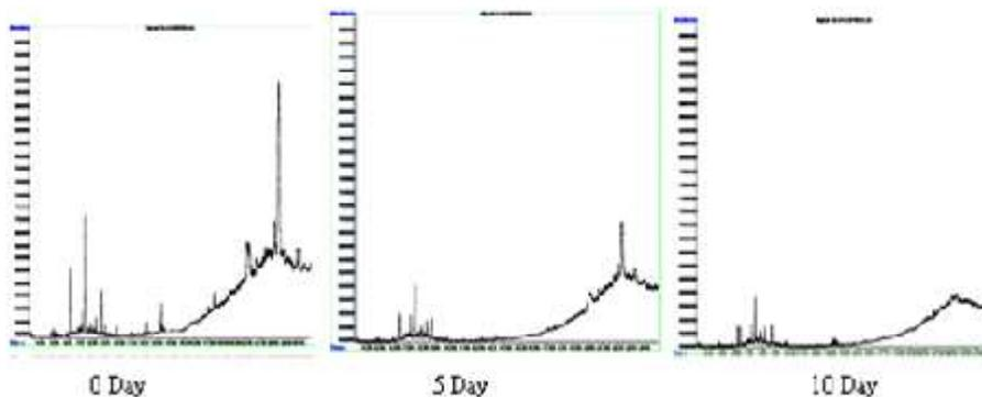
**Fig. 1.** Gas chromatogram of 2T engine oil extracted from M9 medium inoculated with GD<sub>2</sub> strain at 0, 5 and 10 days
