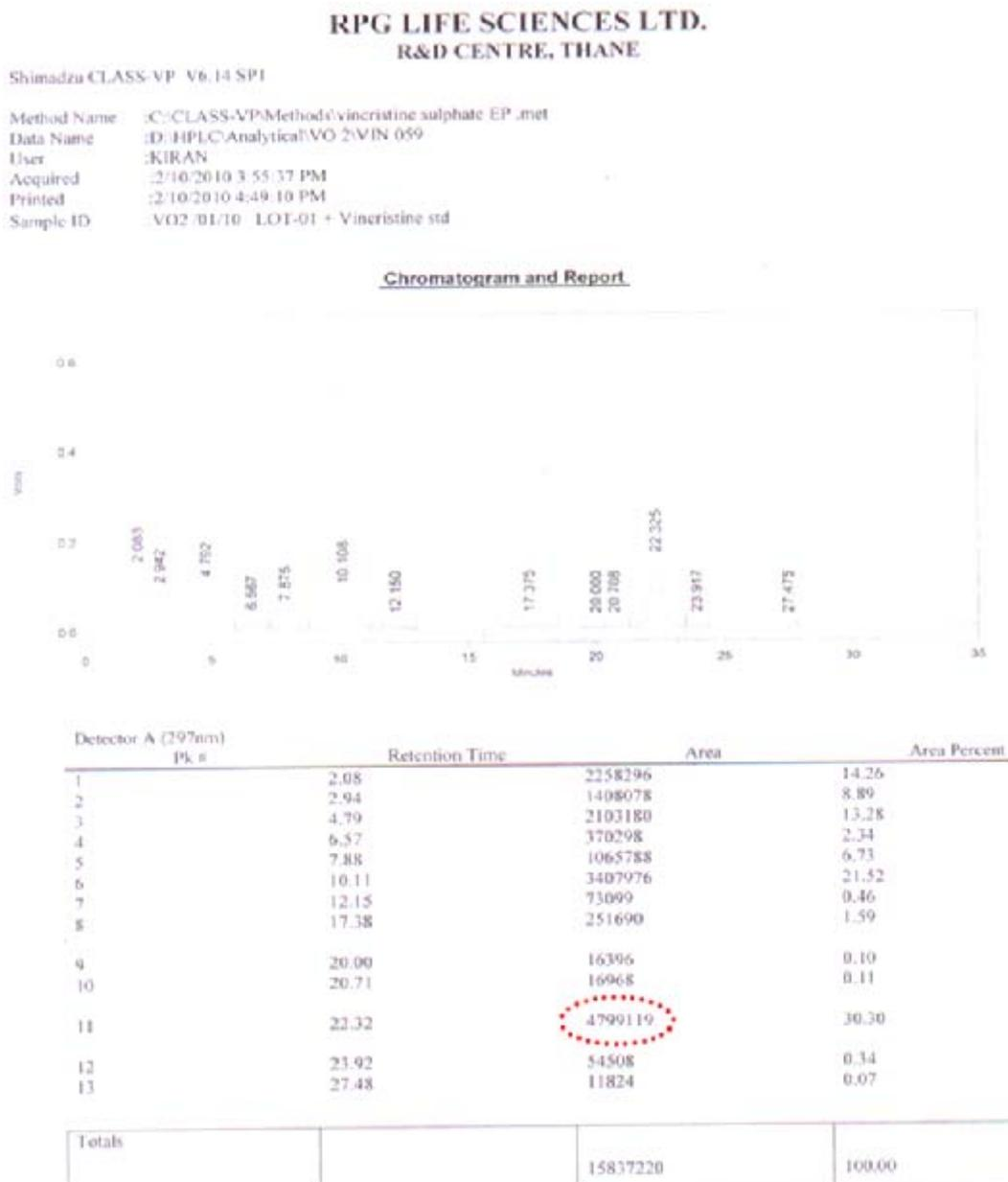
**Fig. 1(b).** Represent the chromatogram of Endophyte RPGLS-03 by HPCL confirming the presence of Vinblastine peak at 22.32 retention time (Minutes)
