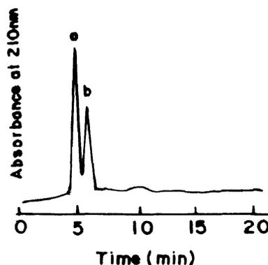
**Fig.4b.** RP-HPLC profile of hydrolysis products of swollen chitin by purified chitinase. 50 µg of purified chitinase in 500 µl of borate buffer pH 9.0 and 1% swollen chitin was incubated for 6 h and boiled for 3 min to stop the reaction followed by centrifugation and lyophilization of the supernatant. The hydrolysis products of swollen chitin were separated on RP-HPLC
