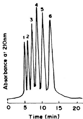
**Fig.4a.** RP-HPLC analysis of reaction products of *Malbranchea chrysosporoidea* chitinase: a. RP-HPLC profile of authentic standards ranging from GlcNAc 1 to GlcNAc 6 peak 1, GlcNAc1; peak 2, GlcNAc2; peak 3, GlcNAc3; peak 4 GlcNAc4; peak 5, GlcNAc5; peak 6, GlcNAc6
