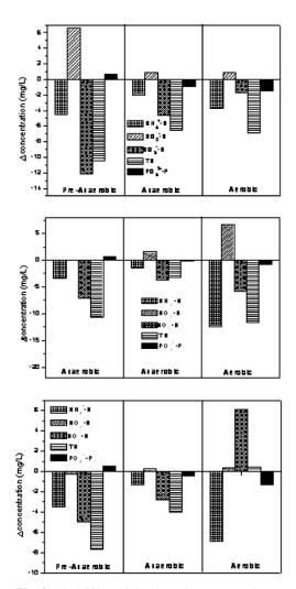
**Fig. 3.** The differential value of  $NH_4^+$ -N,  $NO_2^-$ -N,  $NO_3^-$ -N, TN and  $PO_4^{3-}$ -P concentration at each stage (A: 13#; B: 15#; C: 17#)
