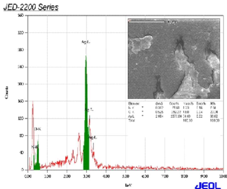
**Fig. 4.** EDS spectra of silver nanoparticles
