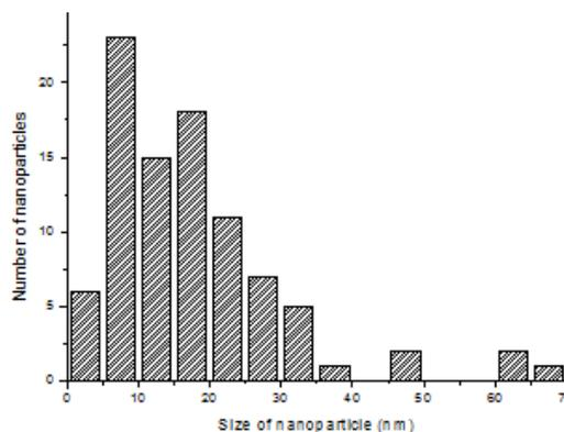
Fig. 7. Histogram for different sizes of biosynthesized silver nanoparticles from TEM images
