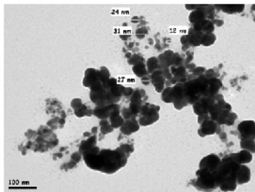
Fig. 6. Images of biosynthesized silver nanoparticles by Transmission Electron Microscopy (TEM)
