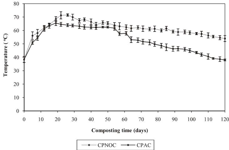
**Fig. 1.** Changes in temperature ( $^\circ\text{C}$ ) during the composting of municipal solid wastes. Values are means of five replicates  $\pm$  standard deviations.
