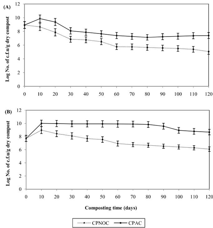
**Fig. 4.** Changes in counts of mesophilic (A) and thermophilic (B) bacteria during the composting of municipal solid wastes. Values are means of three replicates  $\pm$  standard deviations. c.f.u. colony-forming units
