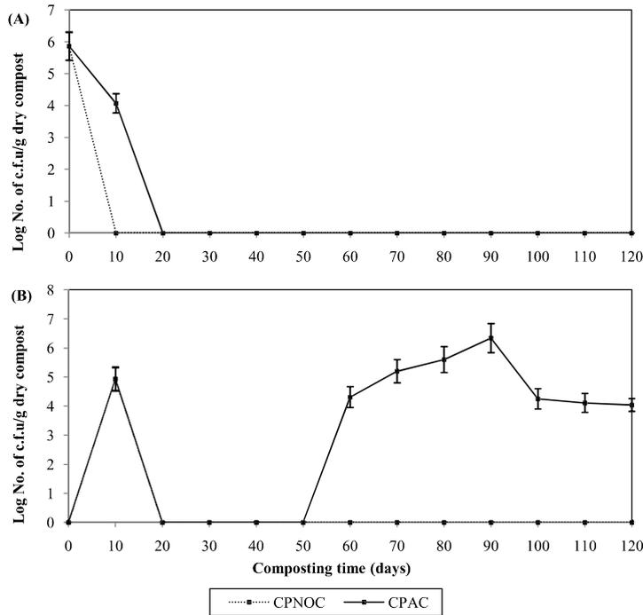
**Fig. 5.** Changes in counts of mesophilic (A) and thermophilic (B) fungi during the composting of municipal solid wastes. Values are means of three replicates  $\pm$  standard deviations. c.f.u. colony-forming units
