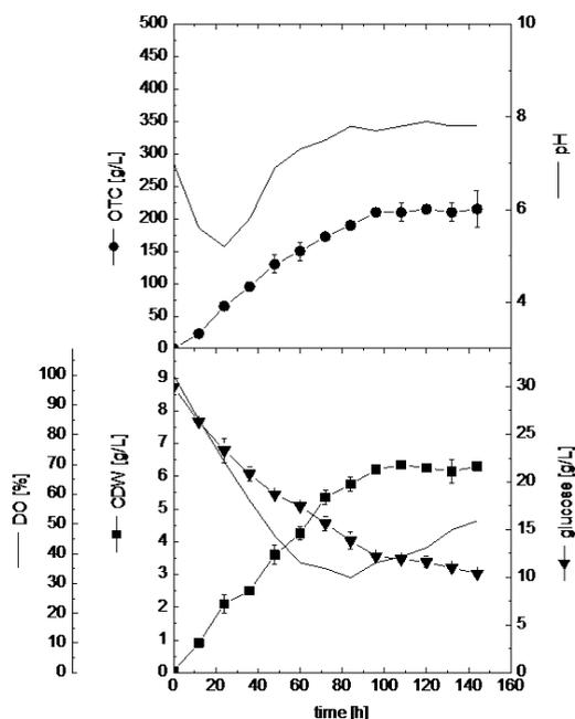
**Fig. 3.** Cell growth, glucose consumption, oxytetracycline production, and pH profile during batch cultivation of *Str. rimosus* in stirred tank bioreactor at 250 rpm, aeration rate 1/v/v/min. and 28 °C.
