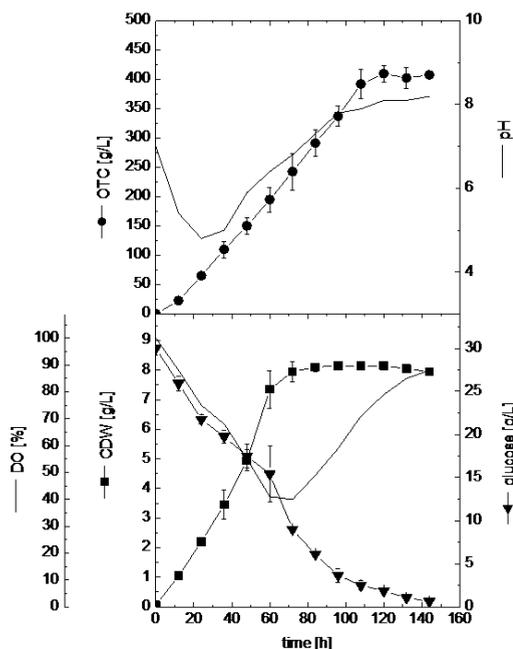
**Fig. 4.** Cell growth, glucose consumption, oxytetracycline production, and pH profile during batch cultivation of *Str. rimosus* in stirred tank bioreactor at 500 rpm, aeration rate 1/v/v/min. and 28°C
