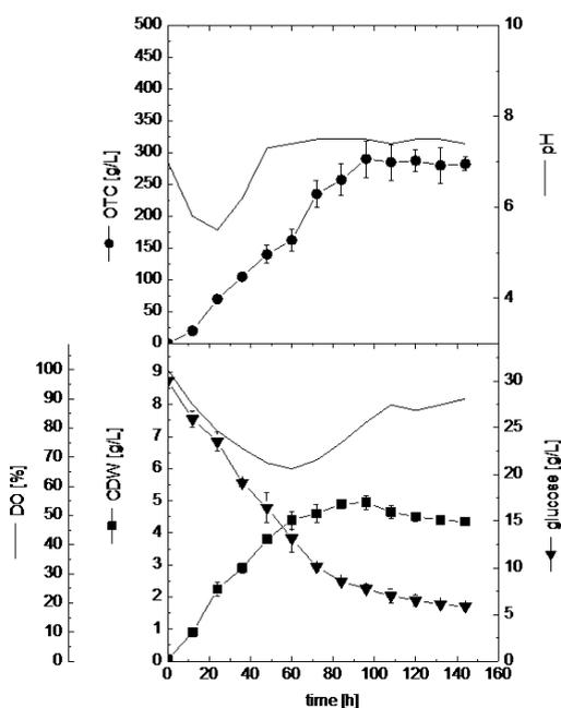
**Fig. 5.** Cell growth, glucose consumption, oxytetracycline production, and pH profile during batch cultivation of *Str. rimosus* in stirred tank bioreactor at 750 rpm, aeration rate 1/v/v/min. and 28°C
