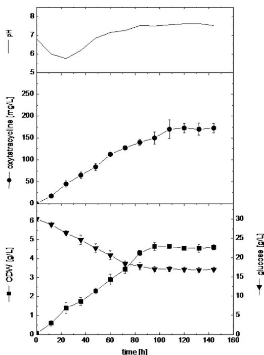
**Fig. 2.** Cell growth, glucose consumption, oxytetracycline production, and pH profile during batch cultivation of *Str. rimosus* in shake flasks at 200 rpm and 28 °C
