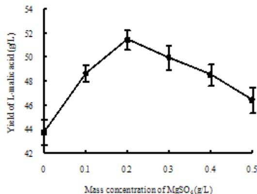
Fig. 5. Effect of mass concentration of  $\text{MgSO}_4$  on the yield of L-malic acid
