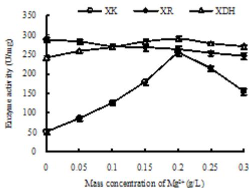
Fig.18. Effect of mass concentration of  $\text{Mg}^{2+}$  on the activity of XR, XDH and XK
