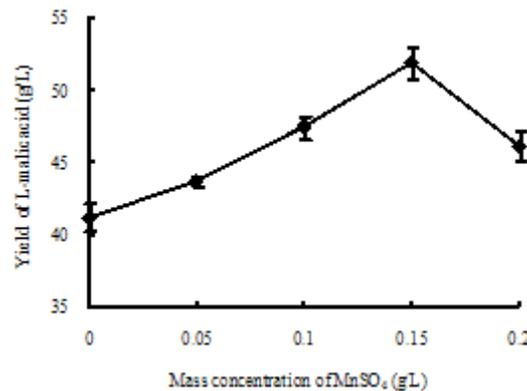
Fig. 6. Effect of mass concentration of  $\text{MnSO}_4 \cdot \text{H}_2\text{O}$  on the yield of L-malic acid
