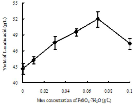
Fig. 7. Effect of mass concentration of  $\text{FeSO}_4 \cdot 7\text{H}_2\text{O}$  on the yield of L-malic acid
