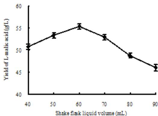
Fig.13. Effect of shake flask liquid volume on yield of L-malic acid
