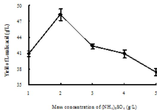
Fig. 2. Effect of concentration of  $(\text{NH}_4)_2\text{SO}_4$  on the yield of L-malic acid
