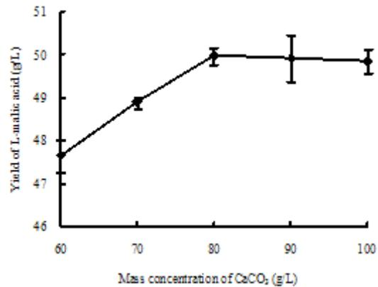
Fig. 8. Effect of mass concentration of  $\text{CaCO}_3$  on the yield of L-malic acid
