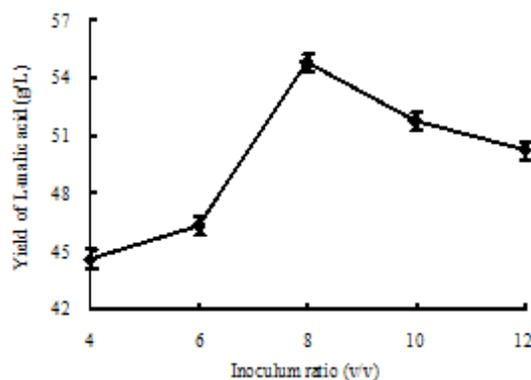
Fig.14. Effect of the inoculum ratio on yield of L-malic acid
