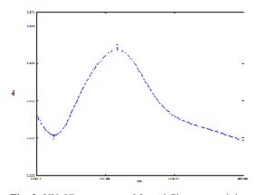
Fig. 2. UV–Vis spectrum of fungal filtrate containing silver nanoparticles synthesized from *Penicillium* spinulosum (MTCC 4952)
