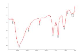
Fig. 3. FTIR spectrum of Silver Nanoparticles synthesized from *Penicillium spinulosun* (MTCC4952)
