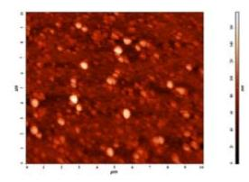
**Fig. 4.** 2D picture of Atomic Force Microscopy (AFM) of silver Nanoparticles synthesized from *Penicillium spinulosum* (MTTC 4952)
