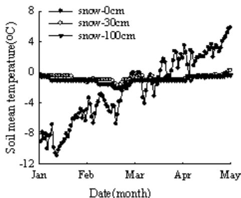
Fig. 1. Daily soil mean temperatures at the depth of 5cm below soil surface under different snow regimes from December 2011 to May 2012
