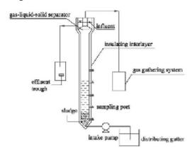
Fig. 1. The structure of UASB reactor
