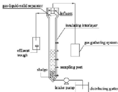
**Fig. 1.** The structure of UASB reactor
