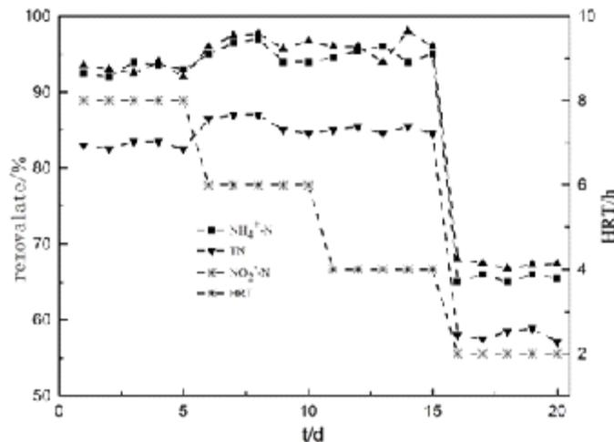
**Fig. 4.** Removal rate vs. HRT for  $\text{NH}_4^+\text{-N}$ ,  $\text{NO}_2^-\text{-N}$  and TN
