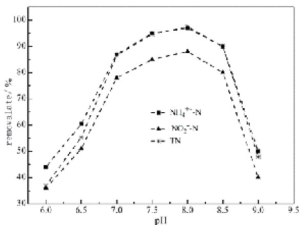
**Fig. 6.** Removal rate vs. pH for  $\text{NH}_4^+\text{-N}$ ,  $\text{NO}_2^-\text{-N}$  and TN
