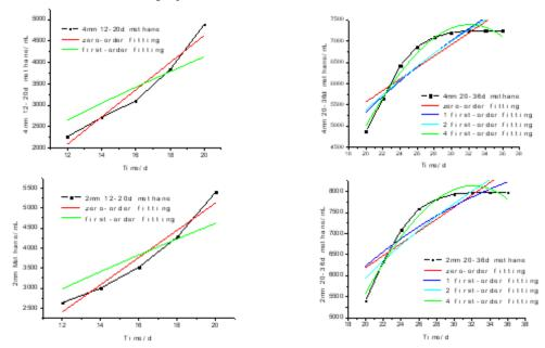
**Fig. 9.** Fitting of different period of accumulative gas production of mixed kitchen wastes J PURE APPL MICROBIO, **8**(2), APRIL 2014.
