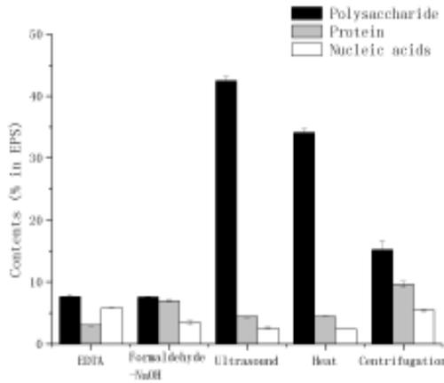
**Fig. 4.** The compositions of mud EPS after 13 days of cultivation with nutrients from different extraction methods
