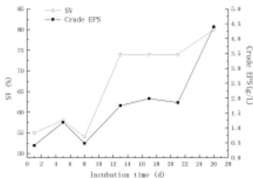
Fig. 2. The variations of settling velocity (SV) and EPS contents of mud during cultivation with nutrients
