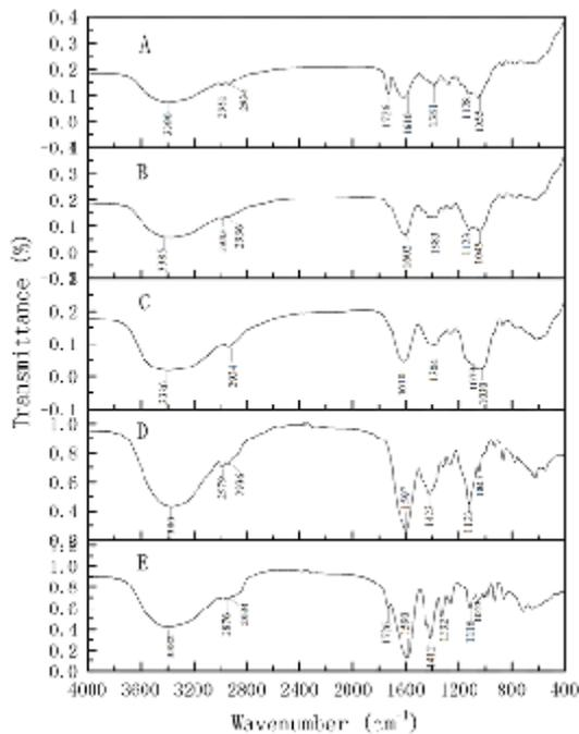
**Fig. 5.** Comparative IR spectra of mud EPS after 13 days of cultivation extracted by different methods. A: Centrifugation; B: Heat; C: Ultrasound; D: Formaldehyde-NaOH; E: EDTA
