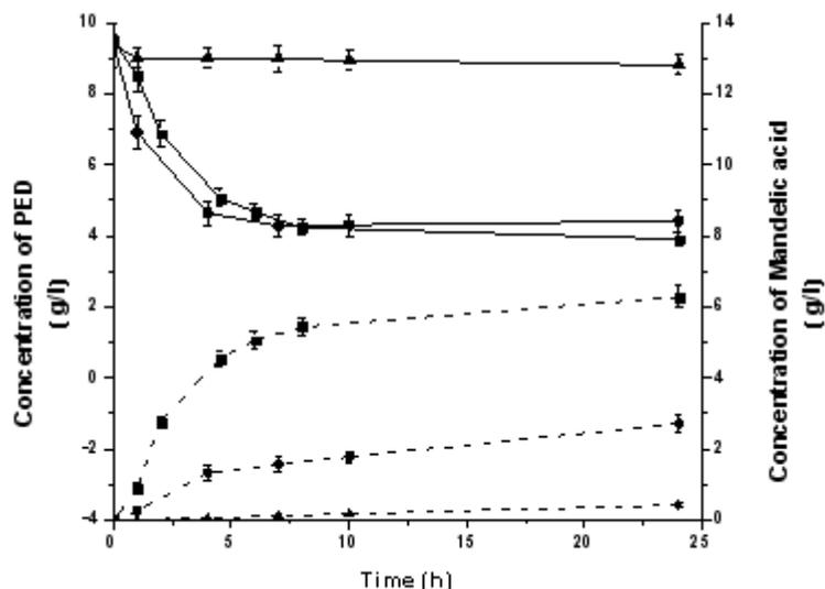
**Fig. 2.** The reaction courses with resting cells of the wild *G. oxydans* strain (■) plus the constructed ADH-knockout (▲) and ALDH-knockout (●) *G. oxydans* strains. The real lines and broken lines respectively represented the changes on concentrations of PED and mandelic acid
