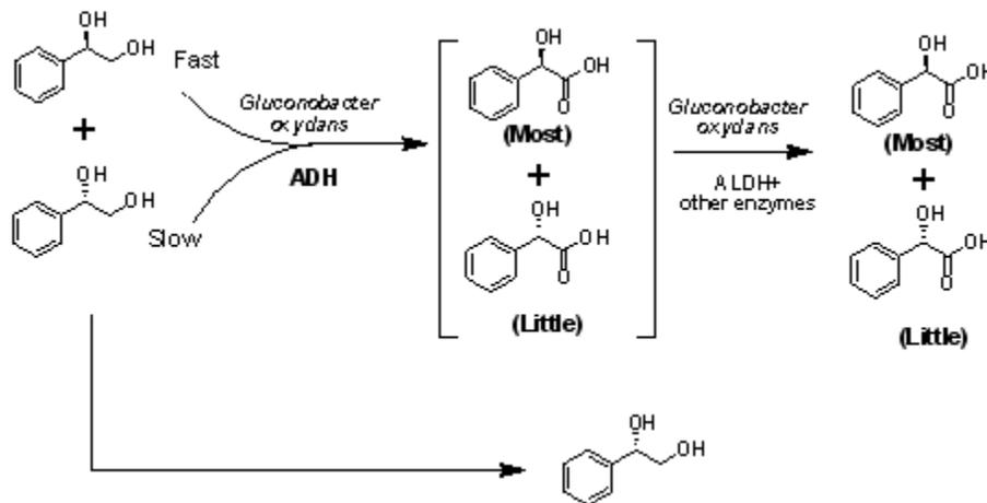
**Scheme 1.** Regio- and Stereo-selective Concurrent Bio-oxidation of racemic PED with Resting Cells of *G. oxydans* DSM2003
