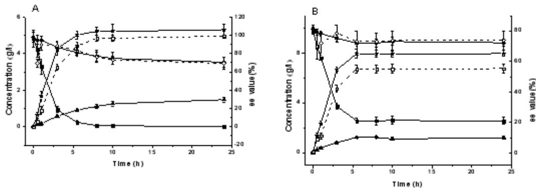
**Fig. 4.** The time curves of reaction at the concentration of substrate 10g/l (A) or 20g/l (B), respectively. The concentrations (real lines) of (R)- (■)/(S)-PED (●) and (R)- (★)/(S)-mandelic acid (▲) were analyzed by HPLC. And then the ee value (broken lines) of (S)-PED (□) and (R)-mandelic acid (◇) were obtained as well. The reactions were carried out under 30°C and pH 6.0.
