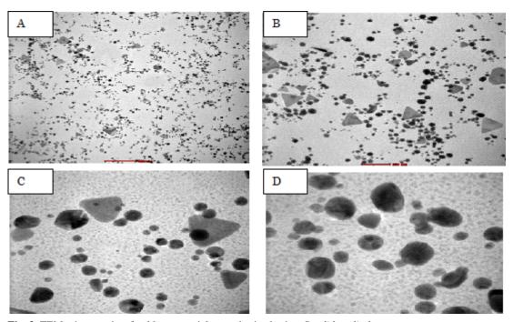
Fig. 3. TEM micrographs of gold nanoparticles synthesized using Candida cylindracea
