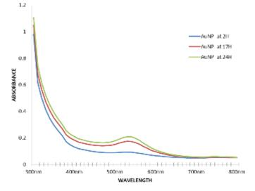
Fig. 2. The UV-Vis spectra of gold nanoparticles formed after different time periods
