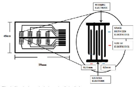
**Fig. 1.** Circuit electrode design using Paint Software J PURE APPL MICROBIO, **8**(SPL. EDN.), MAY 2014.
