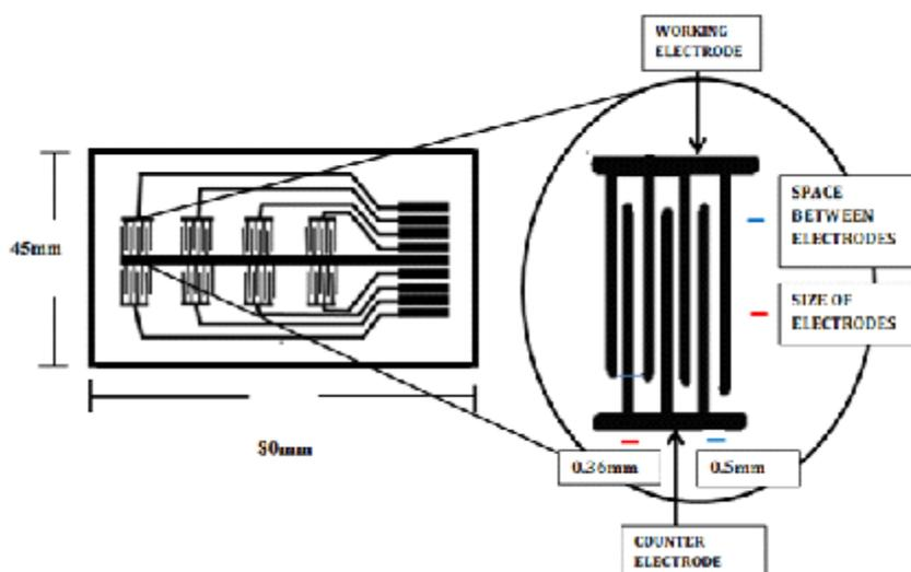
**Fig. 1.** Circuit electrode design using Paint Software
