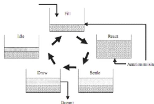
Fig. 1. Typical Cycles in SBR systems<sup>11, 12</sup>
