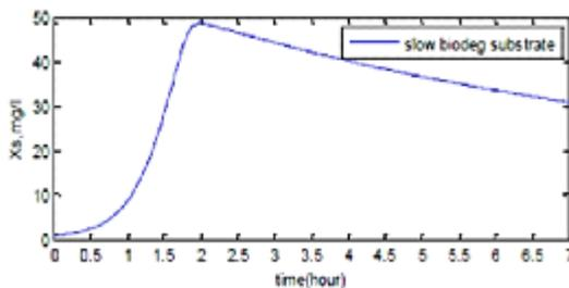
**Fig. 4.** Time profiles of  $X_s$  calculated in optimal conditions for one fill
