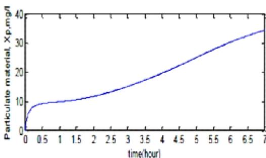
**Fig. 5.** Time profiles of  $X_p$  calculated in optimal conditions for one fill
