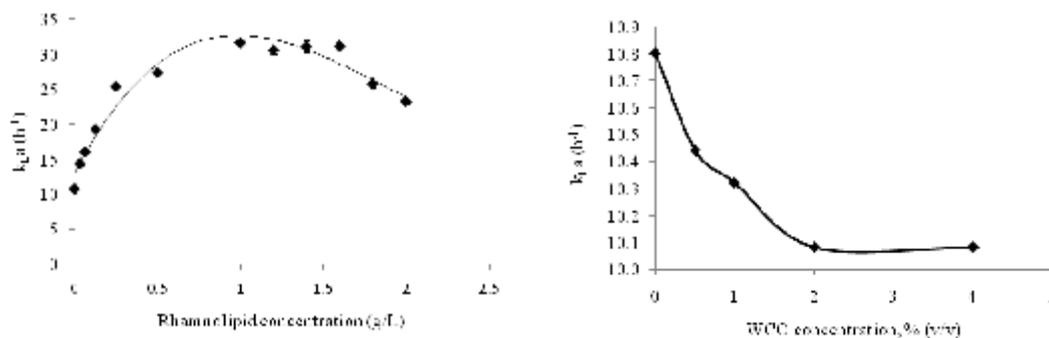
**Fig. 3.** Effect of rhamnolipid and WCO concentration on  $k_L a$
