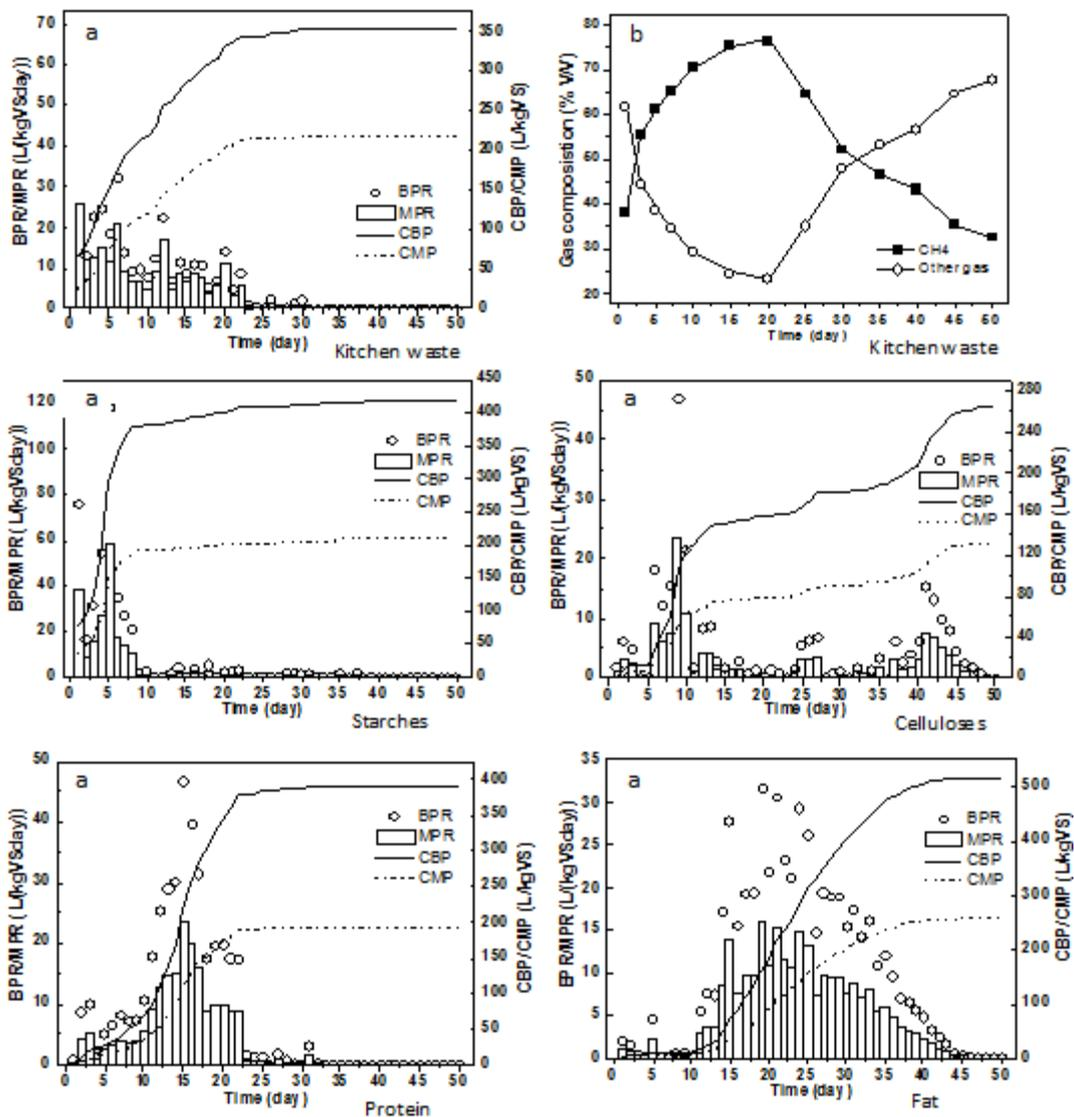
Fig. 2. Evolution of the biogas/CH<sub>4</sub> production rate (BPR/MPR), cumulative biogas/CH<sub>4</sub> production (CBP/CMP) (shown as a) and gas composition (shown as b) for kitchen waste and its components' anaerobic digestions
