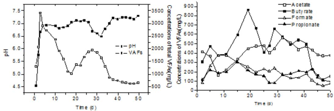
Fig. 1. Evaluation of total VFAs, pH and VFAs for kitchen waste AD
