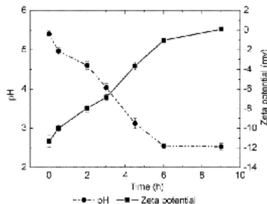
**Fig. 7** Changes of zeta potential and pH of mixed liquor in SBR during one operation cycle.
