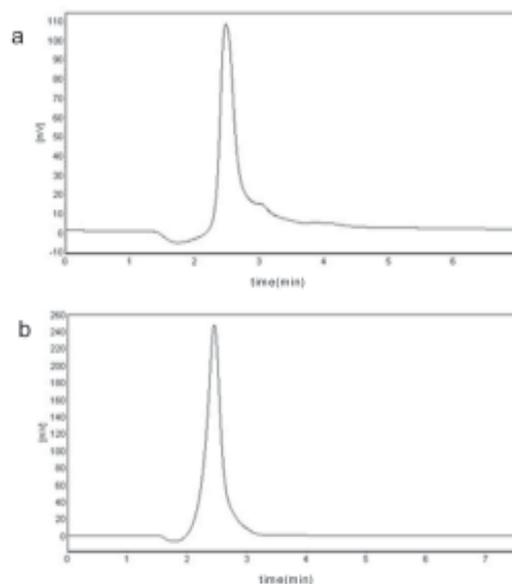
**Fig. 2.** HPLC analysis of poly(3HB-co-4HB) hydrolysis product. (a) 3-HB monomer standard solution, 6 mg/mL. (b) poly(3HB-co-4HB) hydrolysis product by *P. mendocina* DS04-T.
