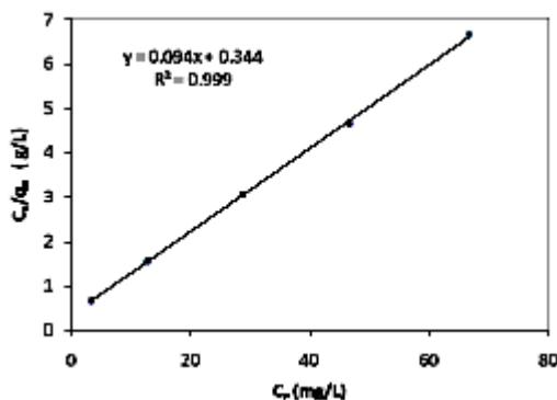
**Fig. 5.** Langmuir adsorption isotherm for Cr(VI) at 0.1 g/ 30 ml of biomass concentration
