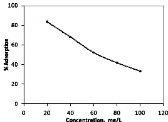
**Fig. 3.** Effect of metal ion concentration on biosorption of Cr(VI) by *Azolla Filiculoides* at 0.1 g/30mL of adsorbent concentration, pH 2 and contact time 100 min.
