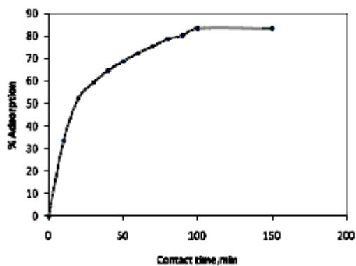
**Fig. 2.** Effect of contact time on adsorption of Cr(VI) by *Azolla Filiculoides* for 20mg/L of metal concentration and 0.1/30mL of adsorbent concentration at pH of 2.
