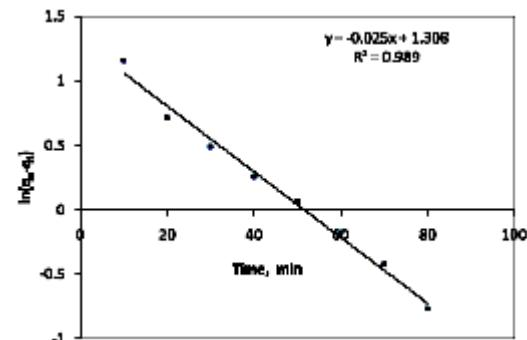
**Fig. 8.** Pseudo first order biosorption of Cr(VI) by *Azolla Filiculoidus* test for 20 mg/L of metal and 0.1 g/ 30 ml of biomass concentration.
