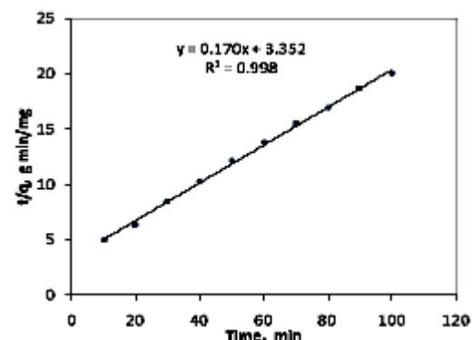
**Fig. 9.** Pseudo second order biosorption of Cr(VI) by sea urchin test for 20 mg/L of metal and 0.1 g/ 30 ml of biomass concentration.
