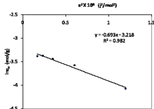
**Fig. 7.** Dubinin– Radushkevich isotherm adsorption isotherm for Cr(VI) at 0.1 g/ 30 ml of biomass concentration
