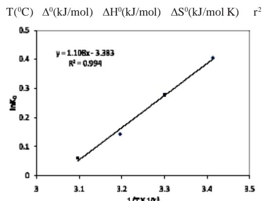
**Fig. 10.** Plot of  $\ln(K_D)$  vs.  $1/T$  for the estimation of thermodynamic parameters for biosorption of Cr(VI) onto *Azolla Filiculoidus* biomass
