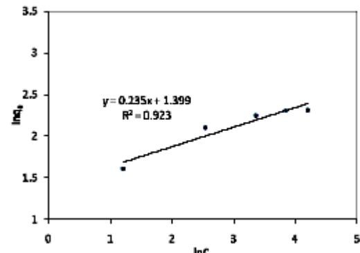
**Fig. 6.** Freundlich adsorption isotherm for Cr(VI) at 0.1 g/ 30 ml of biomass concentration
