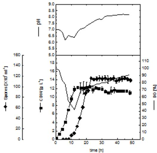
**Fig. 9.** Kinetics of cell growth and spore formation during batch cultivation of *Bti* in 16-L stirred tank bioreactor at an aeration rate of 2.0 v.v<sup>-1</sup>.min<sup>-1</sup>
