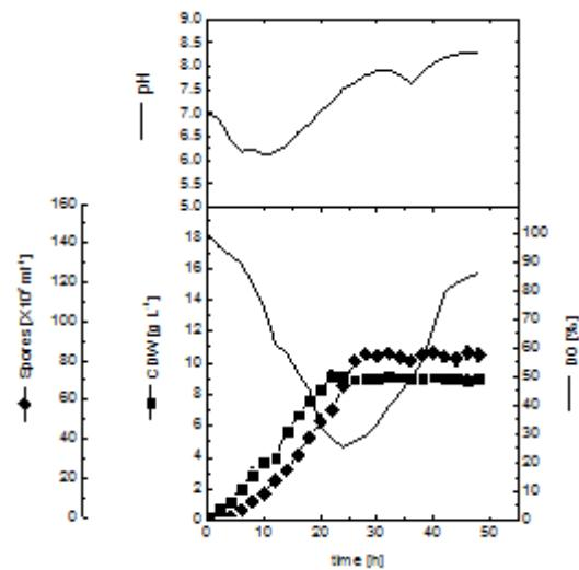
**Fig. 7.** Kinetics of cell growth and spore formation during batch cultivation of *Bti* in 16-L stirred tank bioreactor at an aeration rate of 0.5 v.v<sup>-1</sup>.min<sup>-1</sup>.
