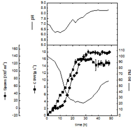
**Fig. 8.** Kinetics of cell growth and spore formation during batch cultivation of *Bti* in 16-L stirred tank bioreactor at an aeration rate of 1.0 v.v<sup>-1</sup>.min<sup>-1</sup>
