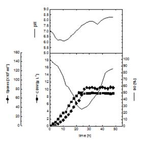
**Fig. 7.** Kinetics of cell growth and spore formation during batch cultivation of *Bti* in 16-L stirred tank bioreactor at an aeration rate of  $0.5 \text{ v.v}^{-1}$ .min<sup>-1</sup>.
