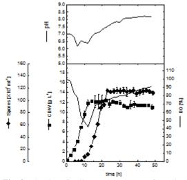
**Fig. 9.** Kinetics of cell growth and spore formation during batch cultivation of *Bti* in 16-L stirred tank bioreactor at an aeration rate of  $2.0 \text{ v.v}^{-1}$ .min<sup>-1</sup>
