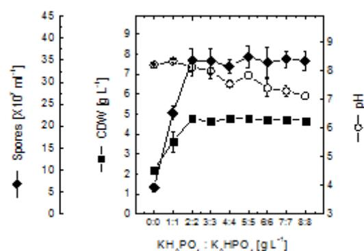
**Fig. 5.** Effect of different initial phosphate concentrations on cell growth, spore production and pH of *B. thuringiensis* var *israelensis*. Cultivations were conducted for 48 hours in shake flasks at 200 rpm and 30°C.
