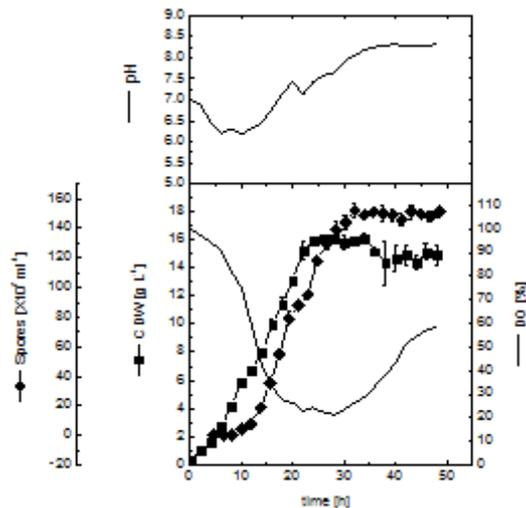
**Fig. 8.** Kinetics of cell growth and spore formation during batch cultivation of *Bti* in 16-L stirred tank bioreactor at an aeration rate of  $1.0 \text{ v.v}^{-1}.\text{min}^{-1}$ .
