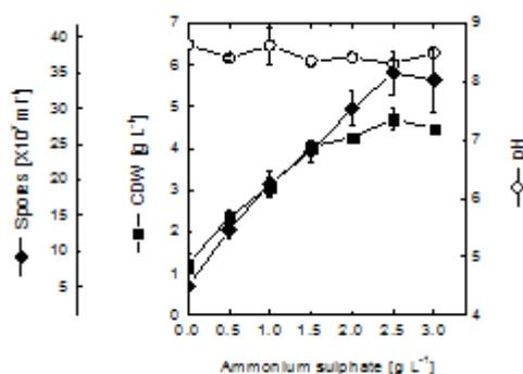
**Fig. 4.** Effect of different initial ammonium sulphate concentrations on cell growth, spore production and pH of *B. thuringiensis* var *israelensis*. Cultivations were conducted for 48 hours in shake flasks at 200 rpm and 30°C
