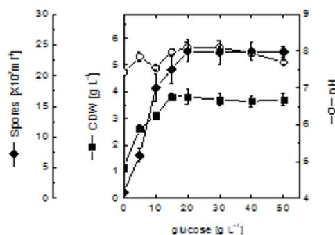
**Fig. 3.** Effect of different initial glucose concentrations on cell growth, spore production and pH of *B. thuringiensis* var *israelensis*. Cultivations were conducted for 48 hours in shake flasks at 200 rpm and 30°C
