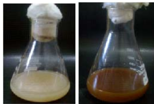
(a) Before addition of \text{AgNO}_3 (b) After addition of \text{AgNO}_3 Fig. 2. Synthesis of silver nanoparticles from Aspergillus flavus
