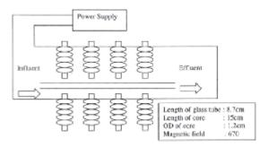
Fig. 2. Schematic Diagram of general magnetic reactor (electromagnets) for sewage treatment<sup>37</sup>
