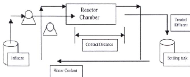
**Fig. 3.** Schematic diagram of a common magnetic wastewater treatment<sup>37</sup>
