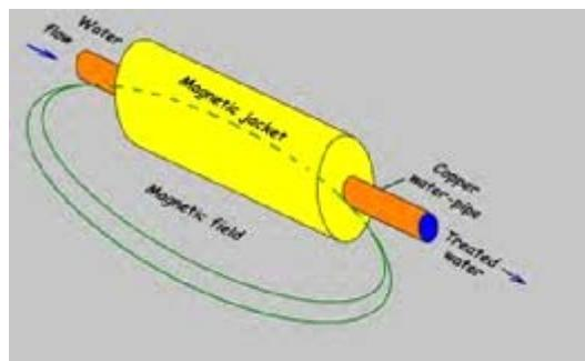
Fig. 1. Schematic diagram of magnetic water system
