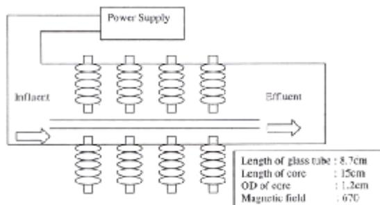
**Fig. 2.** Schematic Diagram of general magnetic reactor (electromagnets) for sewage treatment<sup>37</sup>
