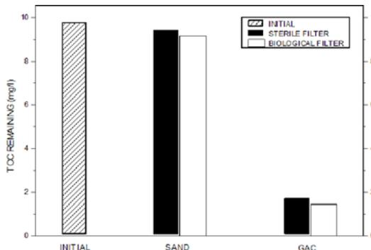
**Fig. 2.** Filtration tests: sand and GAC filters operating on either sterile or biologically active conditions. NOM: commercial humic acids, initial TOC = 9.78 mg/l.
