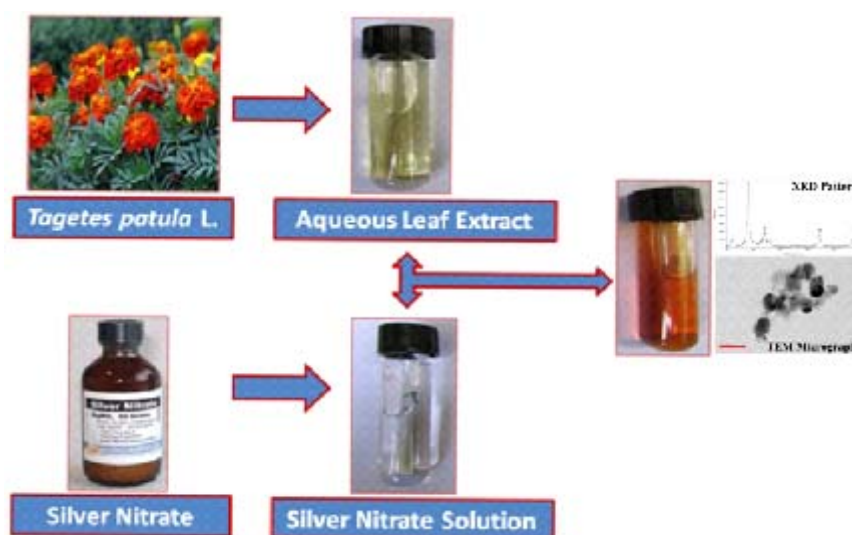
Fig. 1. Schematic representation of synthesis of silver nanoparticles using Tagetes patula L. Leaf extract
