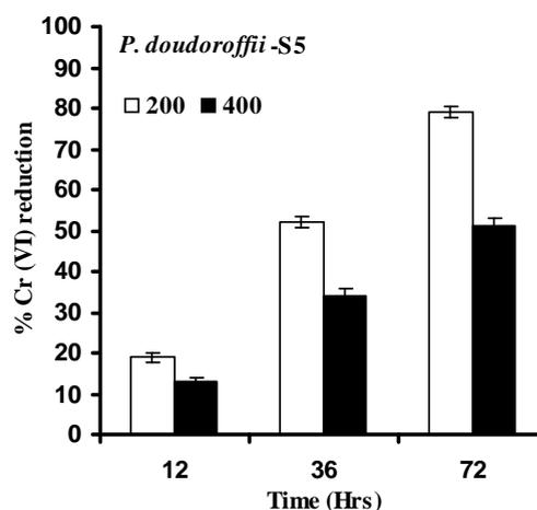
**Fig. 2.** Hexavalent chromium reduction potential of bacterial strains (*B. pumilus*-S4 and *P. doudoroffii*-S5) at different initial Cr(VI) concentration (200 and  $400 \mu\text{g ml}^{-1}$  of  $\text{K}_2\text{CrO}_4$ ) and incubation time (12, 36 and 72 h)
