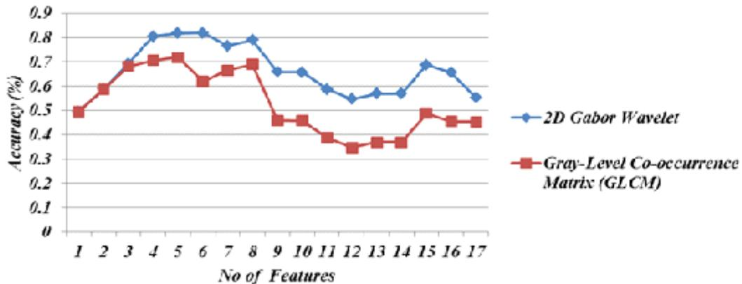
Fig. 3. Comparison of 2D Gabor Wavelet with existing Gray-Level Co-occurrence Matrix method
